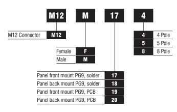
Panel Mount Connectors With Flying Lead (Options and ordering codes)
