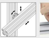
Dismantling: Loosen the tensioning screw, lift the locking strip out of the profile groove and swivel it back. The CLICK-Fastening Set does not need to be taken apart and is immediately ready for use again.
