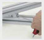
Align the CLICK-Fastening Set and tighten the tensioning screw.
