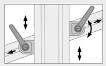
The Angle Clamp Bracket can be used in combination with an Angle Hinge Bracket or a second Angle Clamp Bracket to provide a simple connection between two crossing profiles.
