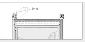
The use of Timing-Belt Reverse Units is a basic requirement for using drive units. The process of opening and closing lifting doors can thus be automated and integrated into manufacturing systems or transport sequences.
