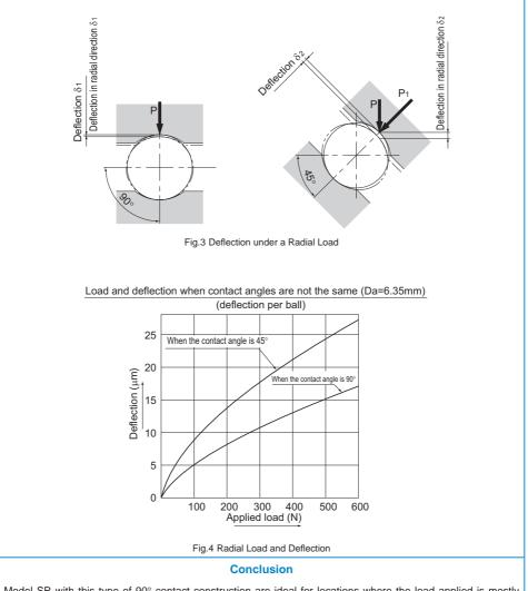
Model SR with this type of 90° contact construction are ideal for locations where the load applied is mostly radial, locations where radial rigidity is required, and locations where accurate motion is demanded in the up, down, left and right directions.
