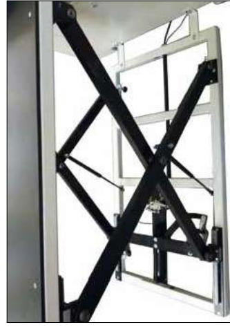
drylin® T rail guides with adjustable clearance change the height of the work table silently and precisely.
