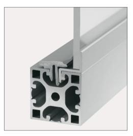
Panel-Clamping Strips consist of a load-bearing aluminium strip in which the panel element is fixed using an elastic plastic strip.
