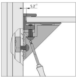
Support Arms X 6-8 are suitable for clamping panel elements 4 to 10 mm thick.
