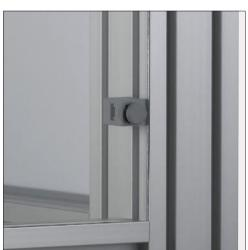
Multiblocks X 8 PA are swivelled into the profile groove at any position. Lightweight metal sheet and panel elements made from Acrylic Glass, Plastic or Compound Material must be provided with a bore at the appropriate location and screwed to the Multiblock.
