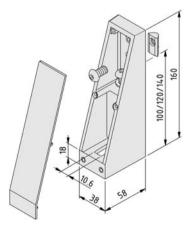
L-Based Foot X 8 adjustable Housing, die-cast aluminium, white aluminium Cap, PA-GF, grey
