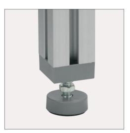
Foot Cap X 8 40x40 light is a plastic cap which is used to cover the end of a Profile X 8 40x40 light if Knuckle Foot X D40 is screwed into the profile's core bore.
