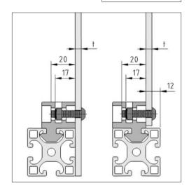
The length of the fastening screw depends on the thickness of the panel element.
