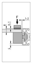
Recommendation for mounting the panel element. The permissible load for Quick Multiblocks 8 PA is  $F=250\ N.$
