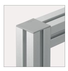
Caps close the end faces of Profiles X 8. They are held in place by a push fit in the Profile's central cavity. The cut edge does not need to be deburred.
