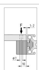
Recommendation for mounting the panel element. The permissible load for Multiblocks X 8 PA is F = 250 N.
