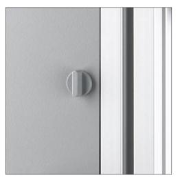
Quick Multiblocks 8 offer the option of fastening a panel element securely in a profile frame in such a way that it can easily be removed. The securing pin is operated either by hand without the need for a tool or using a coin (Quick Multiblock 8 with Slotted Pin).
