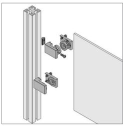
The Panel Clamp is fastened in the groove in Profiles 8 using a screw connection with T-Slot Nut 8. When using the Panel Clamp with Line 6 profiles, a T-Slot Nut 6 St M6 with a Button-Head Screw M6x14 is required. The anti-torsion elements are also to be removed as appropriate for this purpose.
