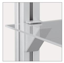
Support Arm X 6-8 is a support for glass shelves or other inherently stable panel elements. Rear clamping of the panel element allows cantilever fastening to a Line 6 or Line 8 profile structure. The form of Support Arm X 6-8 corresponds to the clean contour of profile form X.
