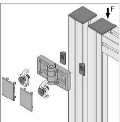
Fastening Hinge X 8 Zn to Line X 8 Profiles. For Profiles with closed grooves, the groove cover is to be removed to insert the T-Slot Nuts and positioning guides.
