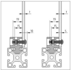
Connection dimensions for Multiblock X 8 PA 0/12 mm.
