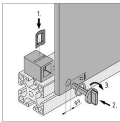
Quick Multiblocks can be used for panel elements of any thickness (up to 8 mm). They can be adapted to the thickness of the panel thanks to two different mounting positions (4 or 8 mm from the edge of the profile). The spring clip is to be inserted in the Quick Multiblock according to the direction in which the load is applied. The concave side of the spring must face the panel and pin. Locking the pin also tightens the spring.
