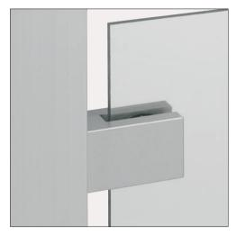
Panel Clamp X 6-8 is a fastener for unframed panels (4-8 mm thick) that does not require any further machining of the panel element. The panel element is held secure by elastic inserts.
