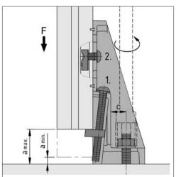
L-Based Foot X 8 adjustable provides a simple method of levelling equipment on uneven floors by means of height adjustment.
