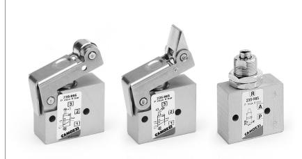
The mechanically operated Series 2 miniature valves with 3-way/2-position normally closed function are available with M5 threaded ports or with an integrated super-rapid fitting for ø 4mm tubes.
