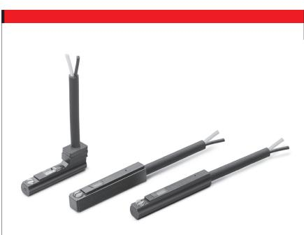
The magnetic proximity switches CSB/CSC define the position of the magnetic piston. When the internal contact is actuated by a magnetic field, the sensors complete an electrical circuit and provide an output signal to actuate directly a solenoid valve or a
